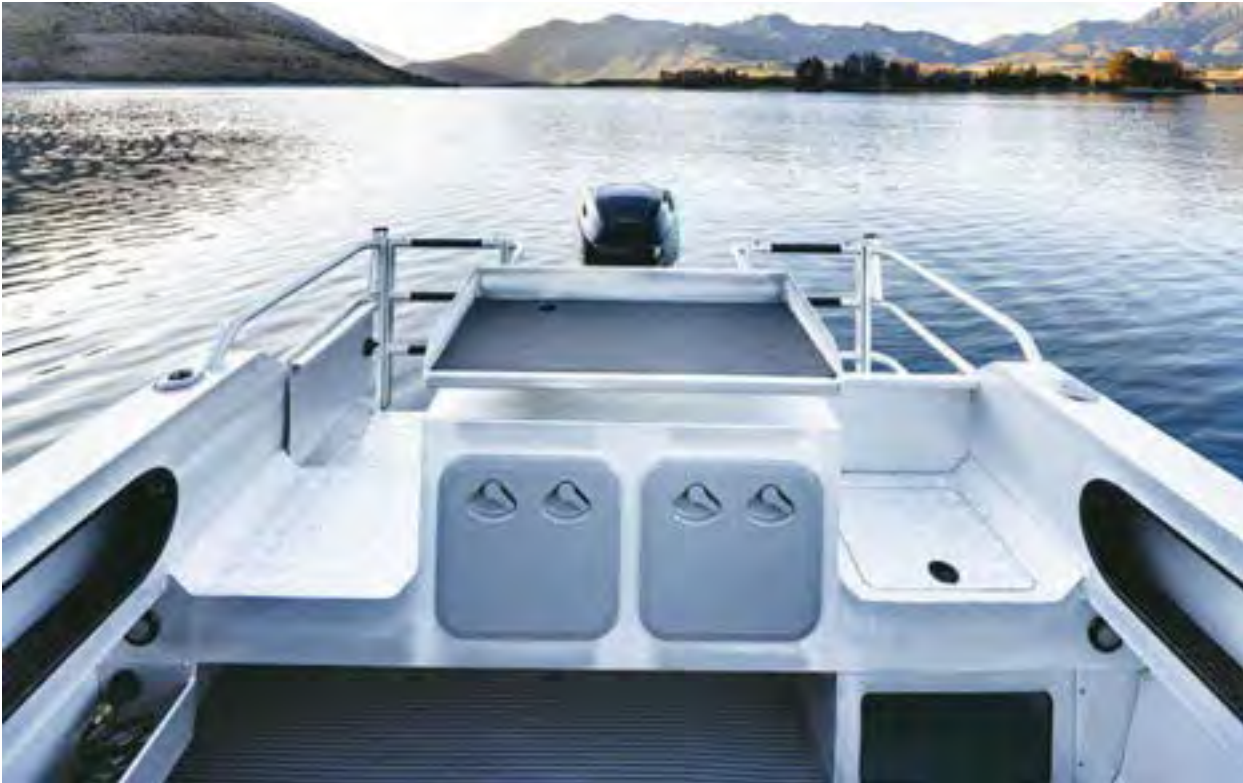
LEFT: LOOKING AFT AT THE TWIN TRANSOM STEPS, THE LARGE CENTRAL BAIT STATION AND LIVE BAIT TANK.
