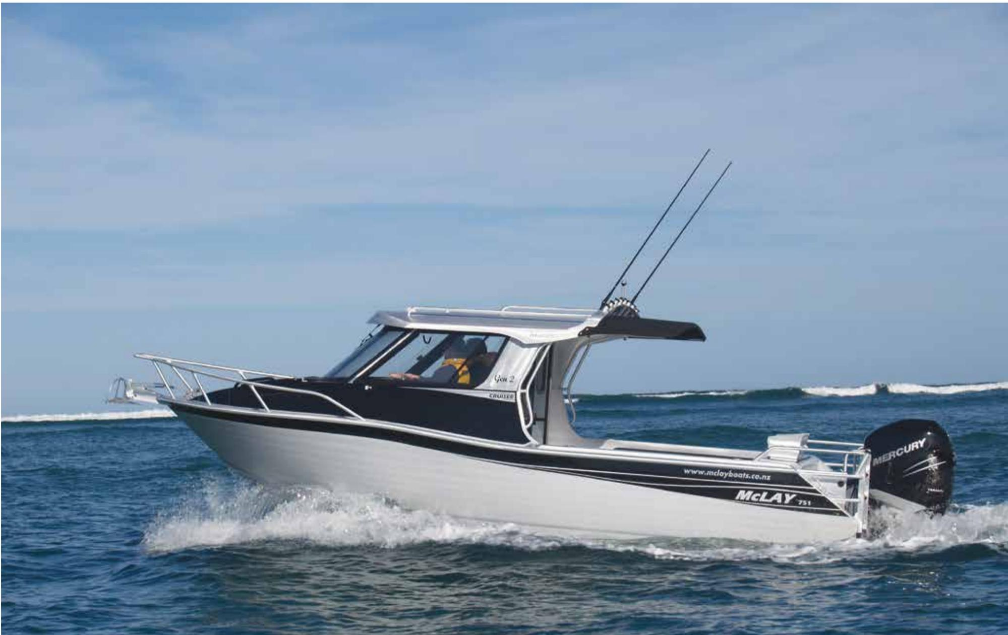
All McLay Boats include air chambers for buoyancy in their hulls and meet the NZ Marine Industry Association and Royal New Zealand Coastguard endorsed Marine Safety CPC build programme requirement that boats must be unsinkable if swamped or capsized, in addition to meeting other key safety and structural criteria.
