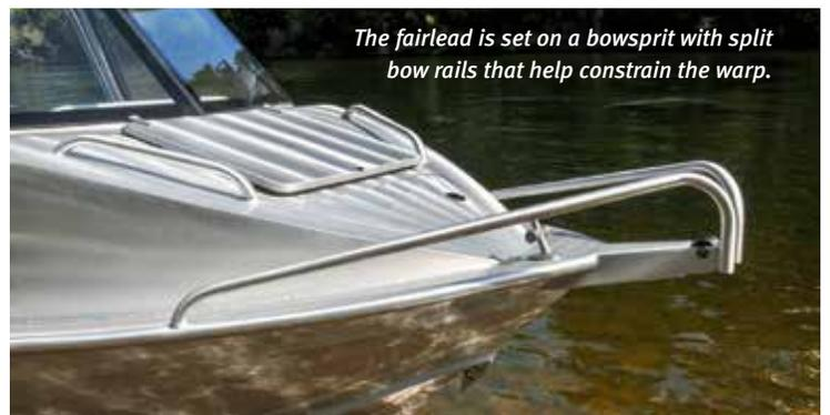
*The fairlead is set on a bowsprit with split bow rails that help constrain the warp.*
