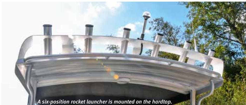
A six-position rocket launcher is mounted on the hardtop.
